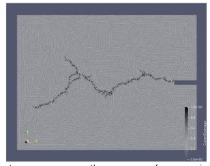
breaking of some of the links created during the compression phase. These ruptures can even cause the appearance of macroscopic cracks such as capping or lamination, which are prohibitive in terms of production [1].
